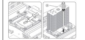
Apply a thin layer of thermal grease onto the CPU surface, and then secure heatink.
