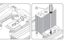
Apply a thin layer of thermal grease onto the CPU surface, and then secure heatink.
