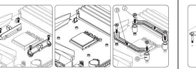
Remove the original AMD plastic retention frame, but keep the backplate; put the standoff on and then secure the AMD bracket with screws.
