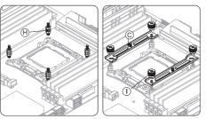
Thread in the LGA20XX screws; put on the brackets and fasten by tightening nuts.
