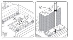
Apply a thin layer of thermal grease onto the CPU surface, and then secure heatink.
