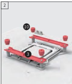
Thread in the LGA20XX standoffs; put on the brackets and fasten by tightening nuts.
